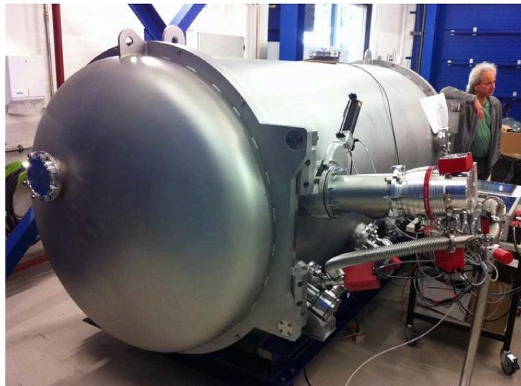
*Figure 4.2: The vacuum chamber for the VIS spectrograph, with an inner diameter and length of 1400 and 3500 mm respectively [37].*
